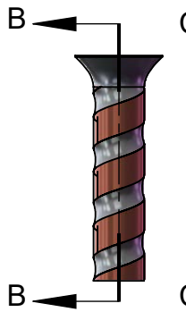
Pb80/Sn20 Cu RIBBON SCALE 15:1
