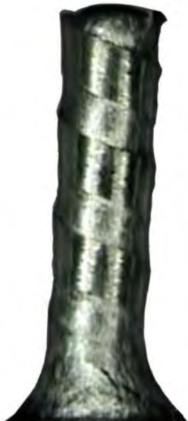
Free end Solder Bump Before Planarizing
