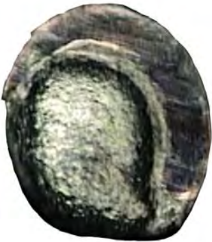
Solder Bump Top of Column
