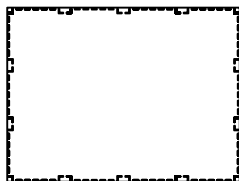
12x16mm 118-PAD 236 BOND WIRES
