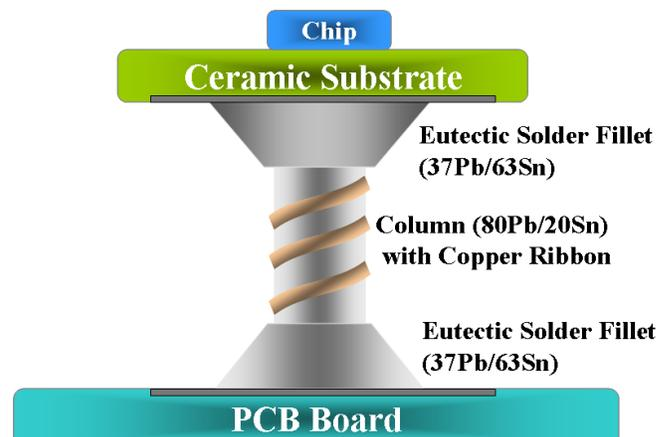
**Figure 1.** Schematic of a Column in a CCGA Package [1]
