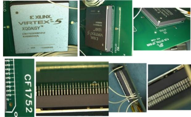
Figure 2. Optical Images of the CCGA Test Board before Thermal Cycling
