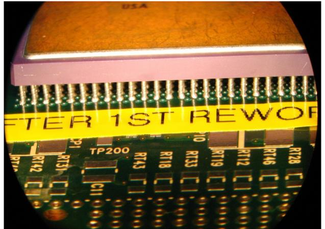
**Figure 18 - Solder joint generated by rework process**
