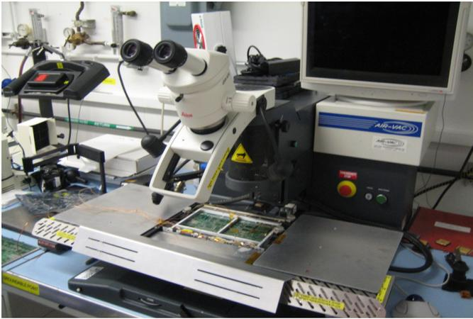
**Figure 14 - Split Vision Rework Station with heat shields installed**
