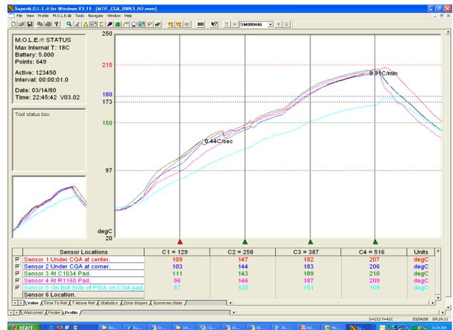
**Figure 8 Graphical representation of thermal profile for Second Series of Temperature Tests**
