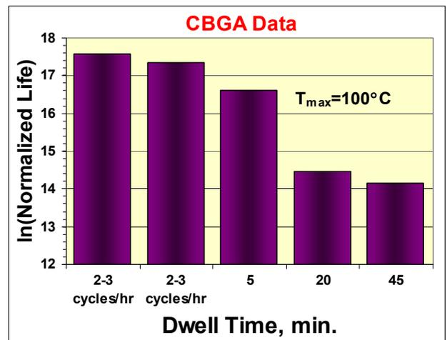
Figure 8. Effect of dwell time on  $N_{50\%}$  life for various ATC with  $T_{\text{max}}=100^\circ\text{C}$ . Note that normalized life (adjusted for substrate dimensions and  $\Delta T$ ) are used to account for variation in test samples and conditions.
