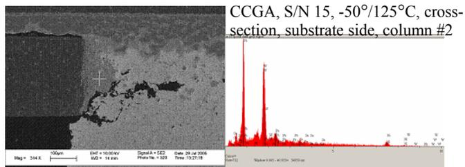
Figure 11. Increased Interposer metallization layer noted.
