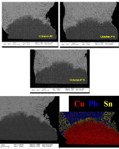
Figure 13. Solder loss and Significant Cu inter-diffusion and IMC formation/growth was noted at board-side solder joints in -50°/125°C ATC (much smaller growth for -50°/75°C ATC).
