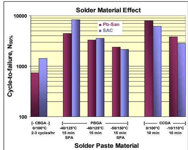
Figure 5. Effect of Solder paste material on cycles-to-failure.
