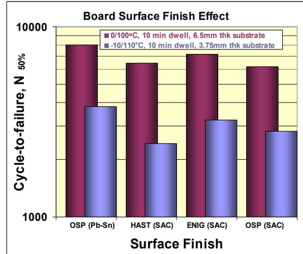
Figure 4. Effect of PCB surface-finish on cycles-to-failure
