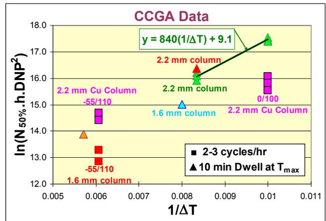
Figure 7. Effect of ATC temperature range on reliability
