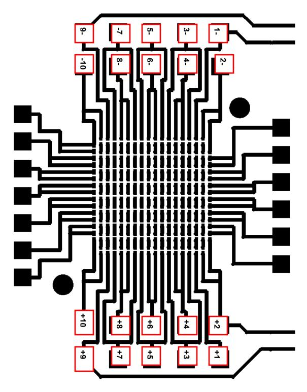
Circuit <u>Before</u> Mounting Flip Chip to PCB
