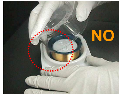
Precaution : Do not replace case cover from the side as this might damage the wire surface.
