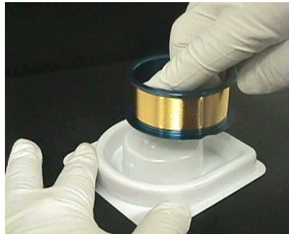
6. When putting the spool back in case, hold the case base and gently put in the spool.
