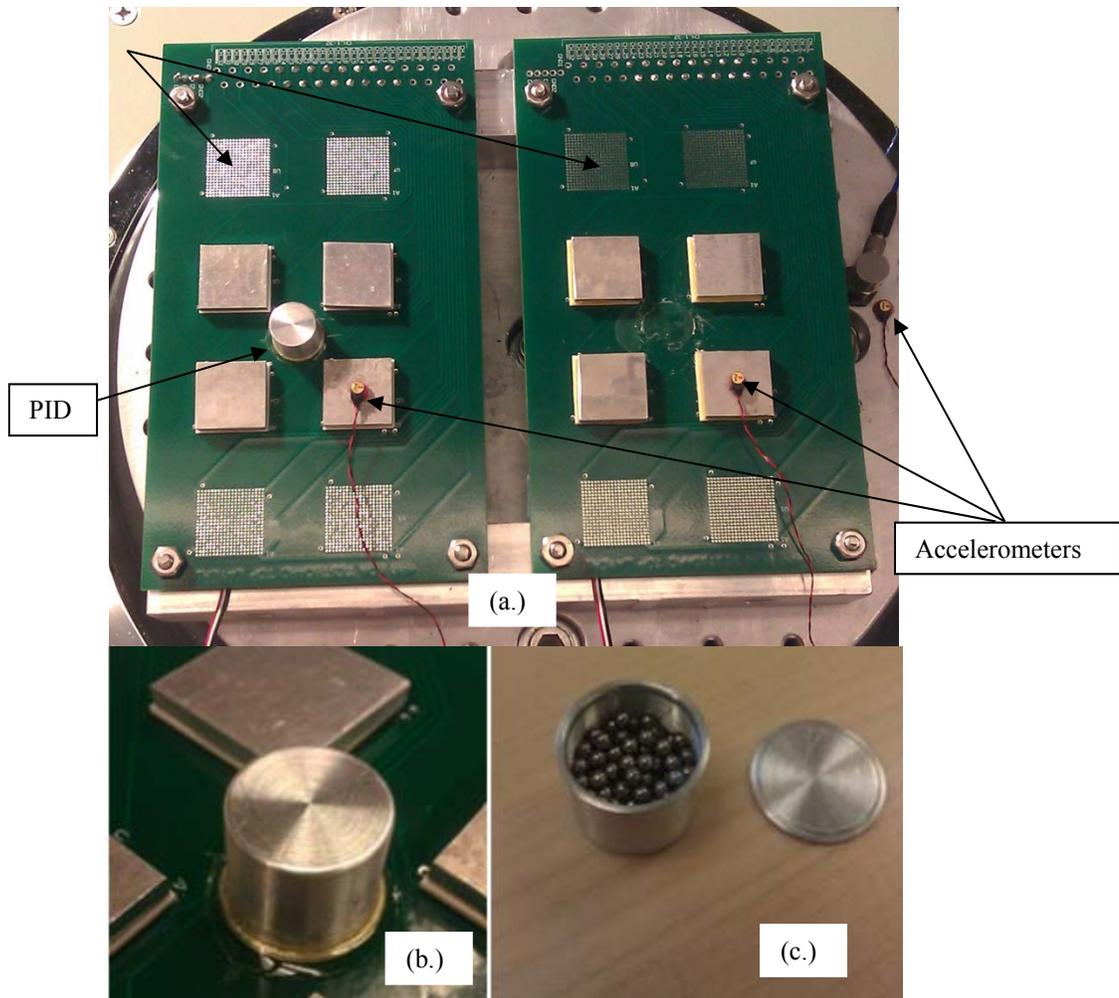
**Figure 5 PWA fatigue test articles (a.) Side by side testing of damped and un-damped boards (b.) Particle damper bonded to board (c.) Open damper filled with 145 Tungsten particles. Cover, (removed here) is in contact with board when installed.**
