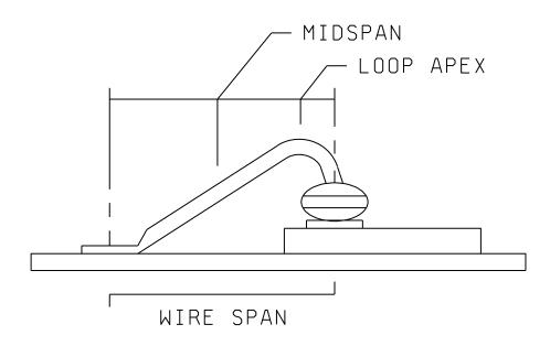
Figure 2011-1. Bond pull hook placement location.
