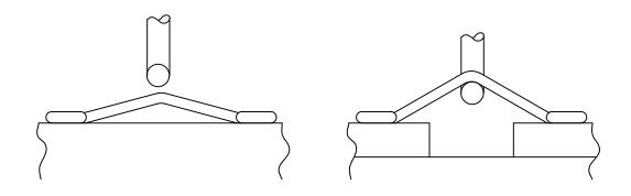
FIGURE 2011-4. Flat loop wire pull testing.
