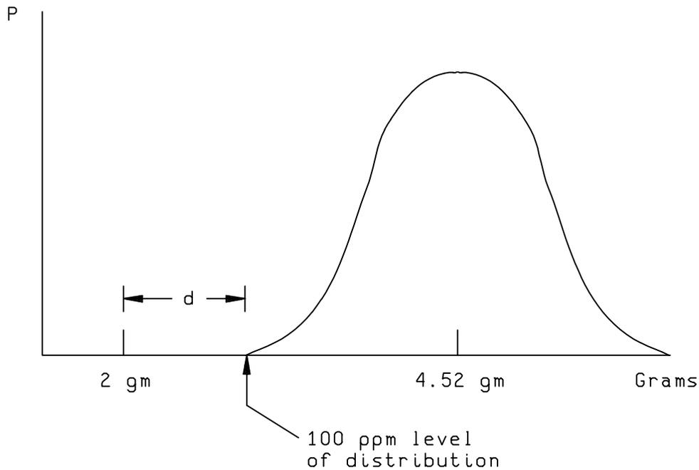
FIGURE 2023-4. Bond strength versus probability.
