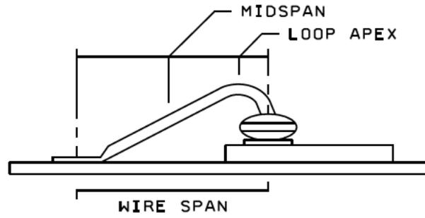
Figure 2023-1. Bond pull hook placement location.
