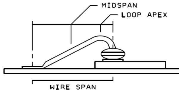
Figure 2023-1. Bond pull hook placement location.
