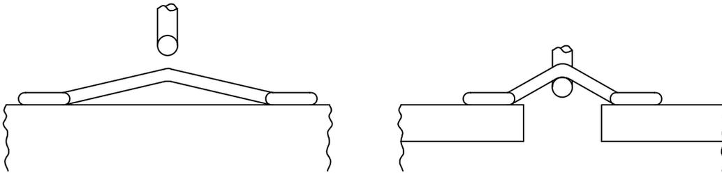
FIGURE 2023-3. Flat loop wire pull testing.
