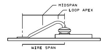
Figure 2023-1. Bond pull hook placement location.
