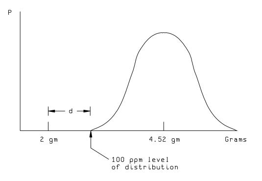
FIGURE 2023-4. Bond strength versus probability.
