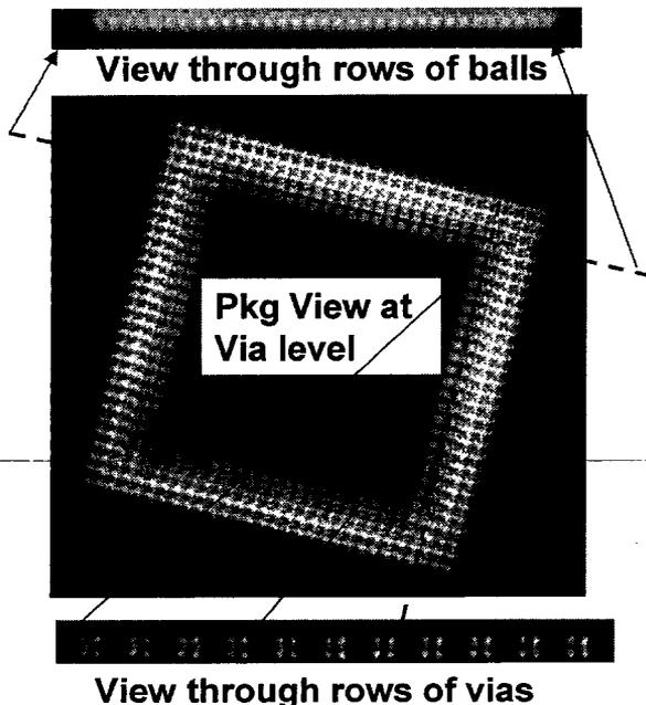
**Figure 5** X-ray photomicrographs of SBGA using a 2D/3D volumetric X-ray system
