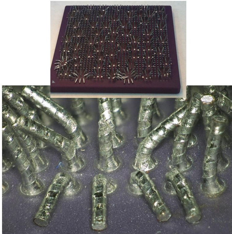
Figure 25. Failure and microstructural changes after 509-hour isothermal aging at 125°C.
